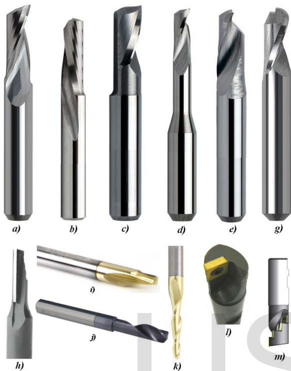
Fig. 1. Types single flute end mill cutters [9],[10],[11]: a) right hand; b) left hand spiral for right hand cutting; c) specially ballance; d) for toric cut; e) engraving; g) with ball nose; h) with right chanel; i) from HSS steel with coating; j) sectional; k) conic extended; l) with carbide replaceable tip; m) high-capacity.
